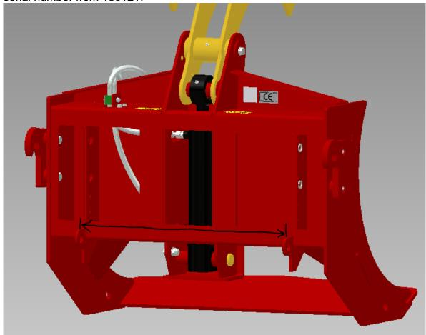
2. Replace Euro attachment with a new type of bracket which expands to the correct distance.
